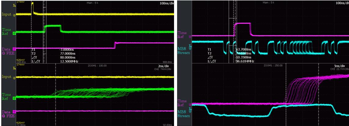
**Figure 11:** Latency and jitter measurement ... (a) **Left:** ... using trigger input. Yellow: Input, Green: Time Reference signal, Purple: Arrival at frontend (on board) (b) **Right:** ... using MBS module. Aqua (blue): MBS data stream (input), Purple: Time Reference. The first falling edge of the MBS data stream starts the trigger message.
