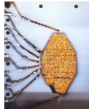
Figure 3.4: The Start/Veto detector in real life. Their height amounts to only 2.5. cm. Source: [Kri08]
