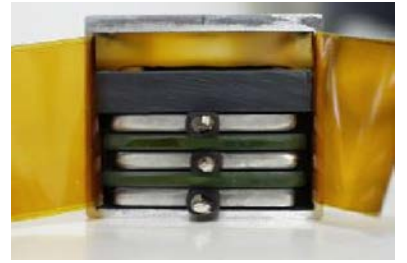
Figure 27: RPC cell with Aluminium-electrodes, glass electrodes, plastic pressure plate, kapton insulation, Aluminium-shielding tube. taken from [22]
