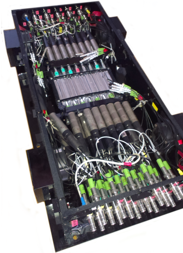
Figure 2.4: Photo of the hodoscope after removing one face of the box.
