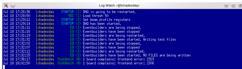
Figure D.4.: The Logfile Monitor shows a log of the most important actions done and errors found within the DAQ system.
