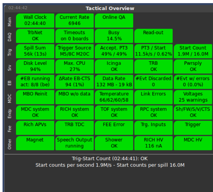
Figure 7.3.: The tactical overview window provides a condensed overview of the status of various aspects of the system. Errors are shown by changing colors.
