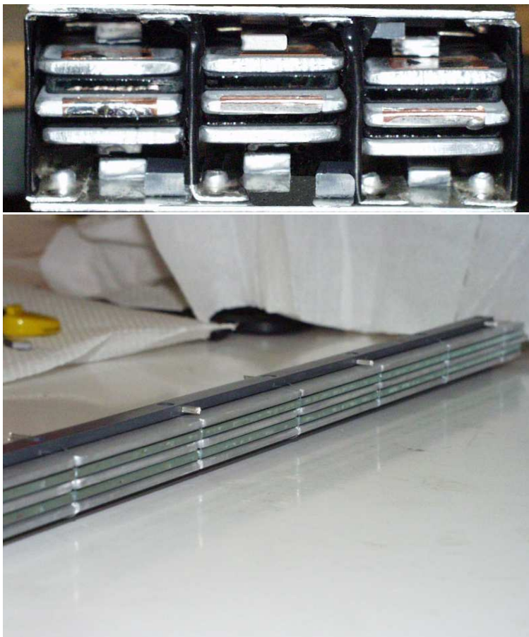
Figure 6.2: Front view of the 3-cell prototype. The left-most cell was replaced by one having glass electrodes (RPC I). In the lower photograph the tRPC cells are shown before placing inside the shielding profile.
