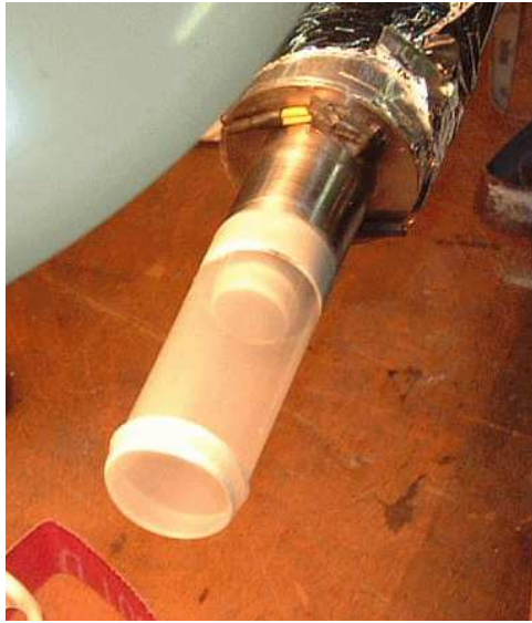
FIG. 2.2 – The liquid hydrogen target vessel with a diameter of 2.5 cm. The entrance window is glued on a stainless steel cylinder.
