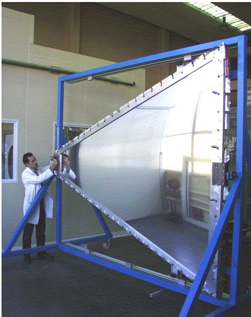
FIG. 2.5 – Left : View of the one HADES Mini-Drift-Chamber, MDC plane IV. Right : An example of measured tension of sense wire of anode plane.
