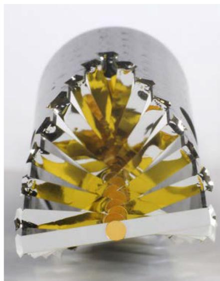
One of the main requirements for the design of the target is to keep the conversion from  $\gamma$  radiation inside the target material into  $e^+e^-$  pairs as low as possible, which is the reason for the segmentation. By maximizing the distance the contribution of conversion in the following segments can be neglected since the  $\gamma$  radiation typically leaves the target material with large
