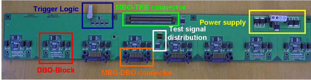
Figure 6.5: Top view of the MBOv1 with 8 \times 4 = 32 channels (size 40 \times 6 = 240 \text{ cm}^2 ).
