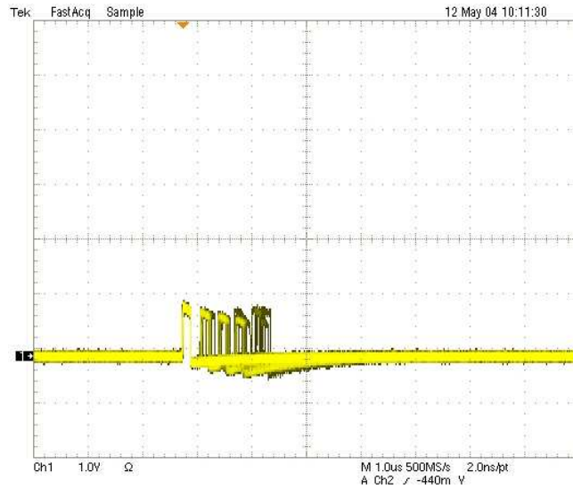
Figure 4.9: Retriggers at the output of the AD96685 discriminator.
