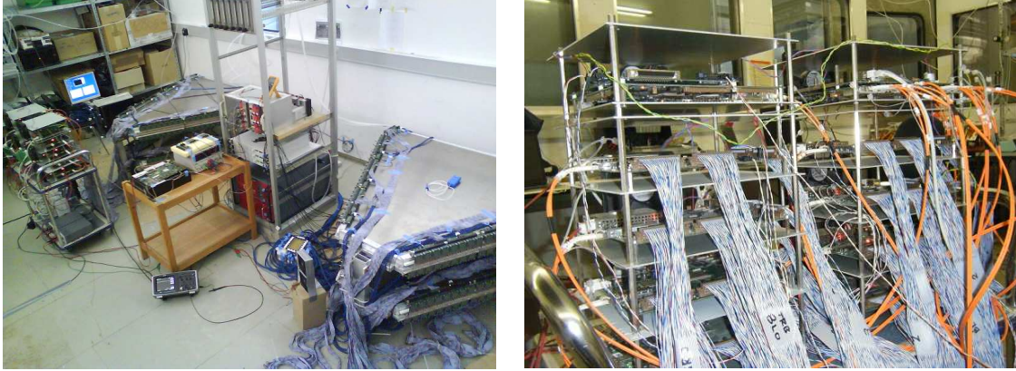
Figure 8.20: Experimental setup of the HADES RPC wall commissioning, showing four assembled sectors with the FEE boards (left) and two stacks of five TRBs each for the DAQ system (right).
