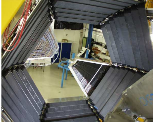
Figure 2.7: A photo of the TOF detectors. The view is from the target area. All six sectors are mounted. In the right bottom corner a part of the magnet is visible. Two sectors of Preshower detector are installed in the center. The right bottom Preshower sector is partially covered by the TOFINO detector (only 3 blocks out of 4 were installed at the time when the photo was made).
