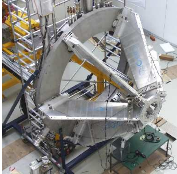
Figure 2.4: Super conducting magnet ILSE composed out of six coils located in the vacuum chambers.
