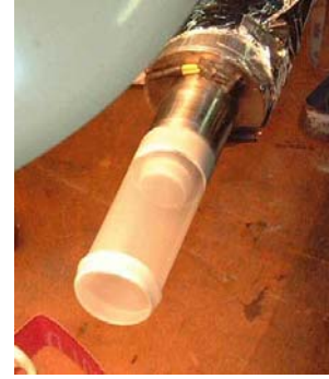
Fig. 24. LH 2 target. The entrance window is glued on a stainless-steel tube with a diameter of 15 mm (visible through the transparent wall of the cell), whereas the target vessel diameter is 25 mm.
