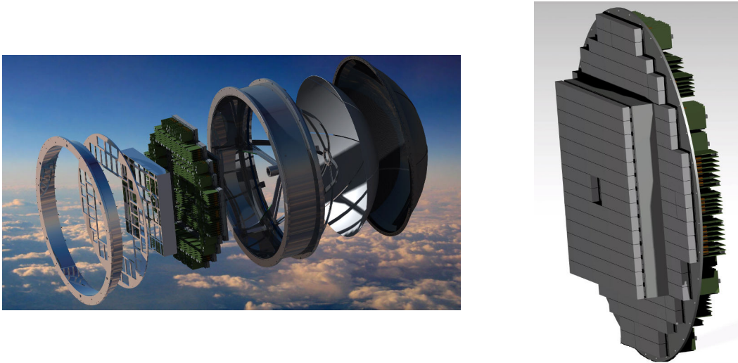
Figure 2.10: Left: Exploded view of the new RICH device after exchange of the gas-filled MWPC photon detector. Right: Front view of the new UV photon detector (active diameter d = 130 cm) with the arrangement of 64-anode photo multiplier tubes.
