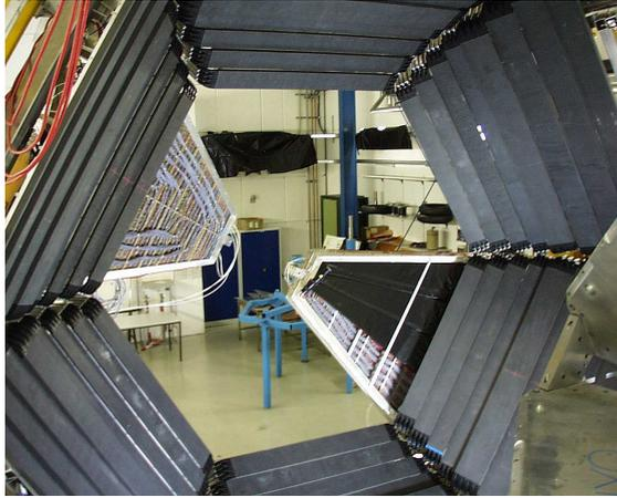
**Figure 1.6:** Picture of the TOF wall detector during its installations on the HADES mechanical support frame. All the six sectors are visible. The two opposite detectors, which are in the center of the picture, are two sectors of the Pre-Shower detector.
