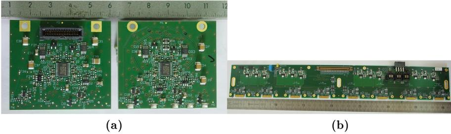
**Figure 3.5:** The HADES RPC Front End Electronics. Left: The four channels DBO (Daughter board). Right: The 32 channels MBO (Mother Board).
