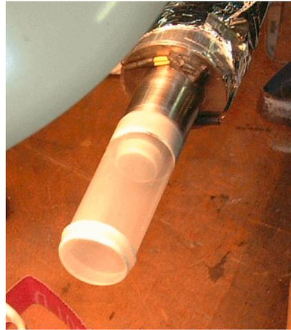
**Figure 4.4:** Photograph of the LH2 target cell.
