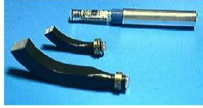
**Figure 4.11:** Photograph of one of the TOF Photomultipliers together with the curved light guides used to couple them to the scintillating rods.
