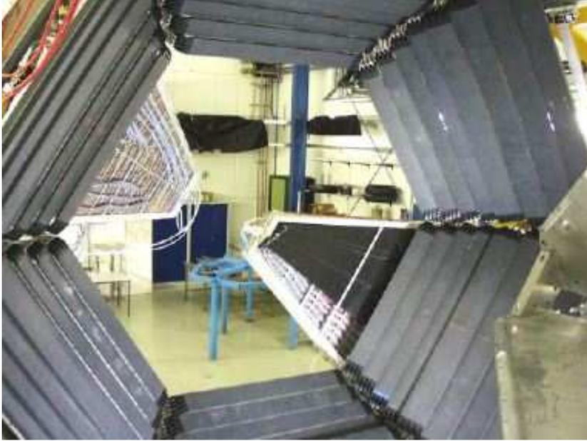
**Figure 4.10:** Photograph of the *Time Of Flight*, **TOF**, detector. The 6 sector symmetry is apparent.
